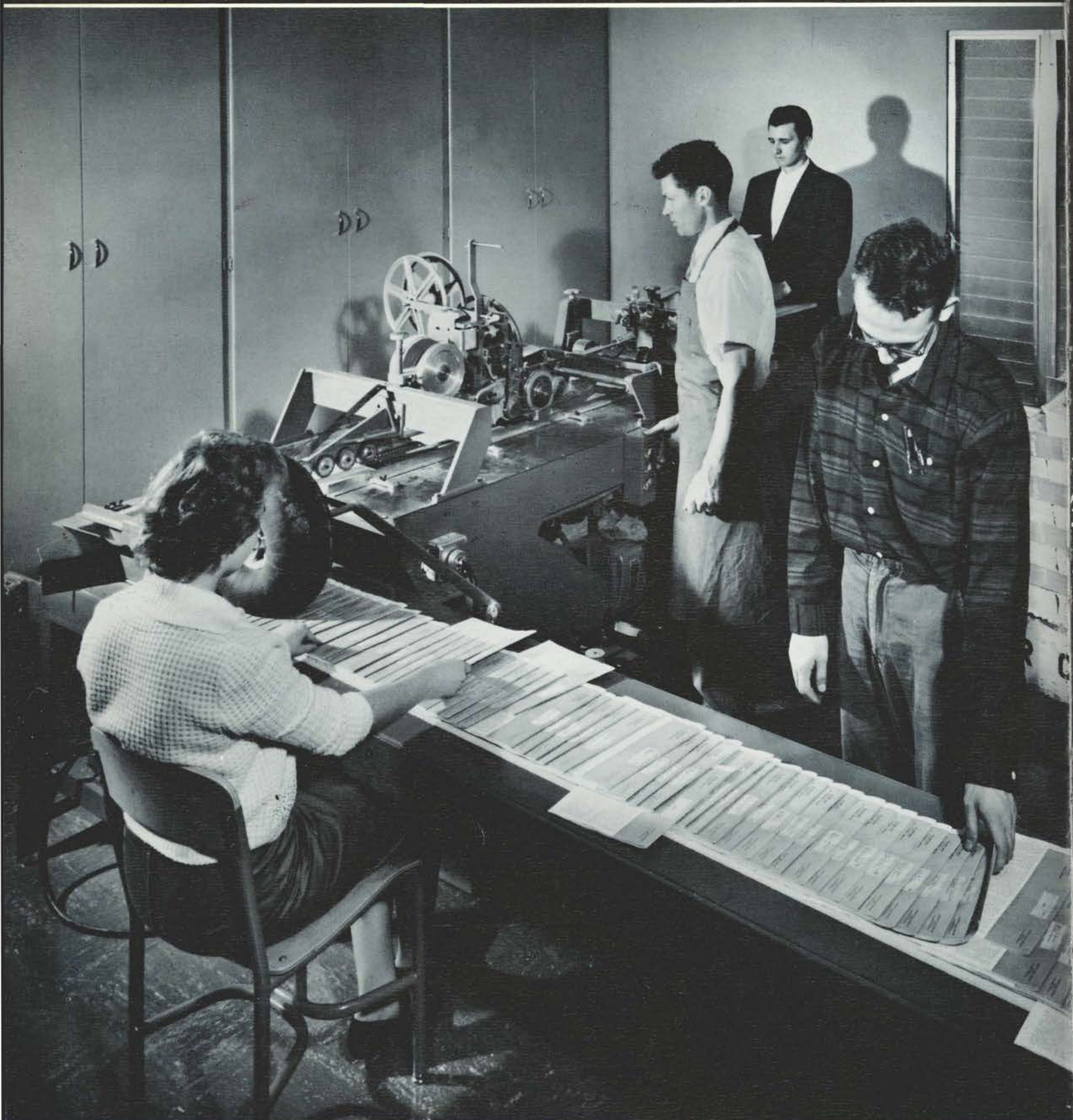
Electronic eyes "read" your address from a perforated card and transcribe it to a moving tape to be applied automatically to your copy of the Plain Truth as is being done by this machine.
