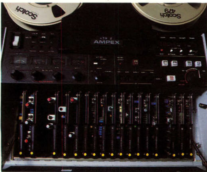
In keeping pace with the television industry's transformation from two-inch to one-inch tape, Ambassador's Television Production studios now utilize a new one-inch Ampex video tape recorder.
