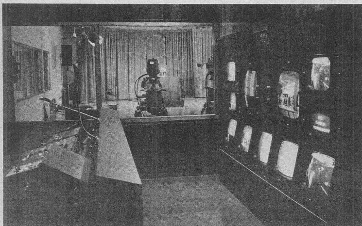
FROM THE CONTROL BOOTH — Looking out into the studio from the control booth, we view the cameras zooming in on a color picture to ready the program for proper color. From the control booth, the picture can be monitored on the monitor bank, right, and controlled by the control panel on the left. [Photo by Howard Clark]
