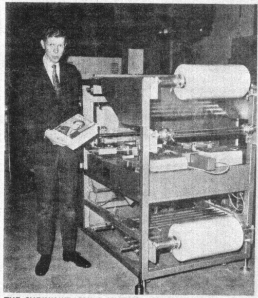
THE SHRINK-WRAPPING SYSTEM — Mr. David Silcox stands by the shrink-wrapping system, which meets the expanding needs of The Plain Truth's newsstand project.
